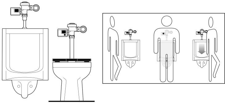
The AutoFlush™ sends out a continuous infrared beam that is reflected back by the presence of a person in front of the urinal or toilet. "Object Lock" technology differentiates between someone walking past the unit or actually using the fixture.
