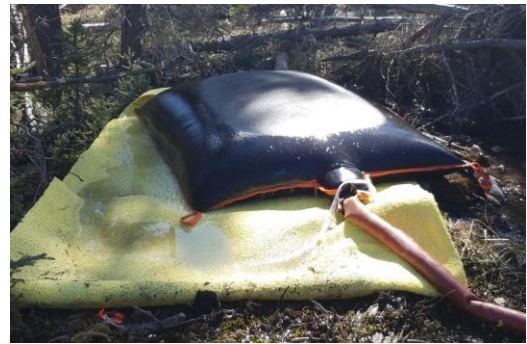
Grey water filtration device.
