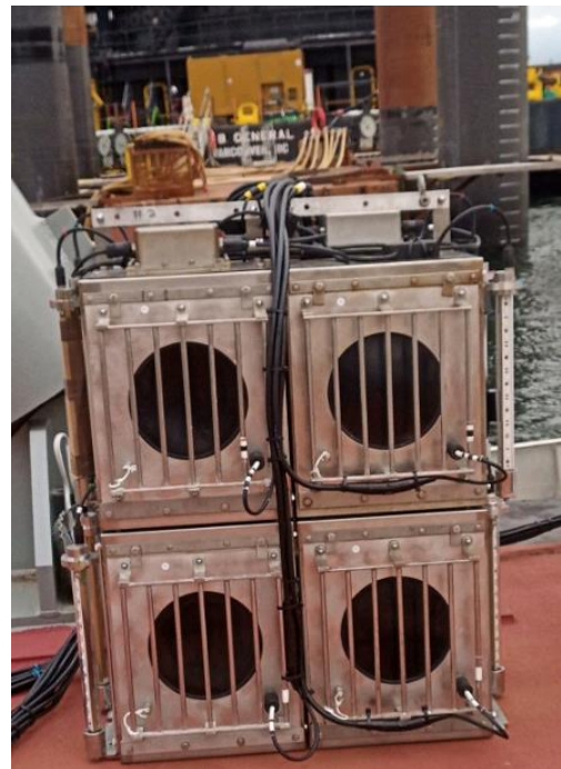
Fish Acoustic Deterrent System before underwater deployment.
