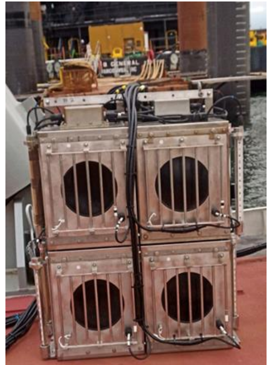
Fish Acoustic Deterrent System before underwater deployment.
