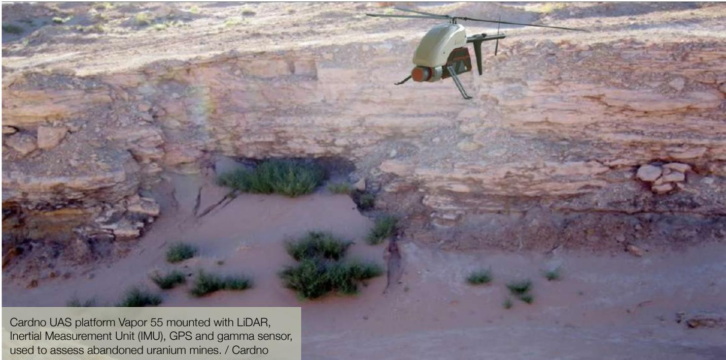
Cardno UAS platform Vapor 55 mounted with LiDAR, Inertial Measurement Unit (IMU), GPS and gamma sensor, used to assess abandoned uranium mines. / Cardno
