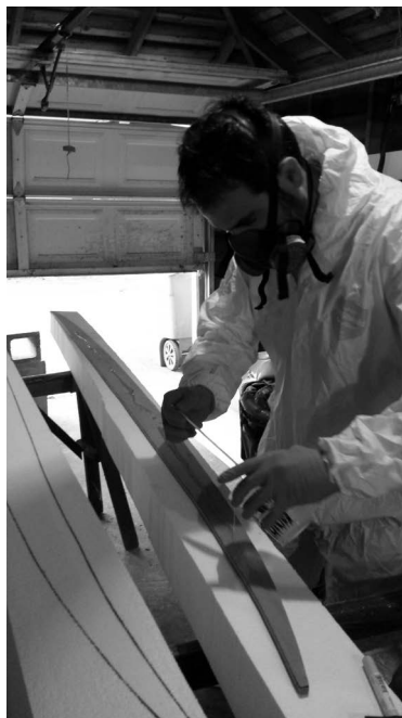
Gluing in the red cedar stringer between the blocks of foam and of course wearing the proper PPE! Safety first! Photo: Annika Lennarz
