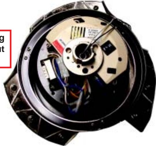
Disconnect the motor and receiver pin connectors. Also disconnect the light circuit connectors from receiver. The receiver can now be removed and replaced with the new receiver.
