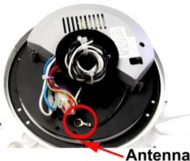
Disconnect the motor and receiver pin connectors. Also disconnect the light circuit connectors and antenna. The receiver can now be removed and replaced with the new receiver.
