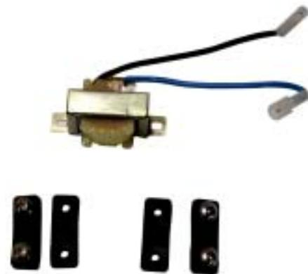
NOTE : Reconnect the choke coil the same way as it was blue wire connector from receiver to blue connector on choke coil and black wire from choke coil to wire connector from motor that may be blue or black.
