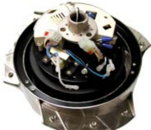
Install new receiver and secure with screws that were removed from the receiver that was replaced secure antenna to mounting plate. Reconnect the motor, receiver and light circuit connectors. Make sure that dip switch settings on receiver are matched to hand held transmitter before replacing top cover.
