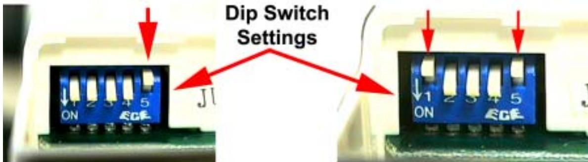
Note : For fans to operate properly dip switch number five must be set in the off or up position. Notice arrow and on position for setting guide.
