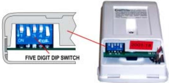
— W 42 rear view dip switch location shown with 9 volt Alkaline battery removed.
