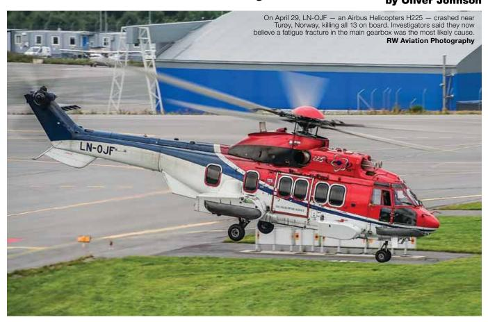
Norwegian investigators have said a fatigue fracture in the main gearbox (MGB) was the most likely cause of the fatal Airbus Helicopters H225 crash near Turøy, Norway, on April 29, and said the fracture propagated in a manner unlikely to be detected by existing mandatory or supplementary systems.
