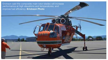
Erickson Inc. and Helicopter Transport Services (HTS) have announced the first flight of advanced composite main rotor blades for the S-64 Aircrane and CH-54 Skycrane.
