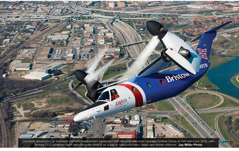
an H-tail with rudders — and the AW609, which has a rudderless T-tail and relies solely on differential collective pitch for yaw control in high-speed flight. Moreover, in 2013, Leonardo substantially modified the shape of the aircraft's rear fuselage and vertical fin, the original design for which had been carefully developed through wind tunnel testing to compensate for the T-tail's low inherent directional stability.
