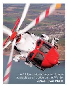
option on the AW189 and follows certification of the limited ice protection system (LIPS) in September
