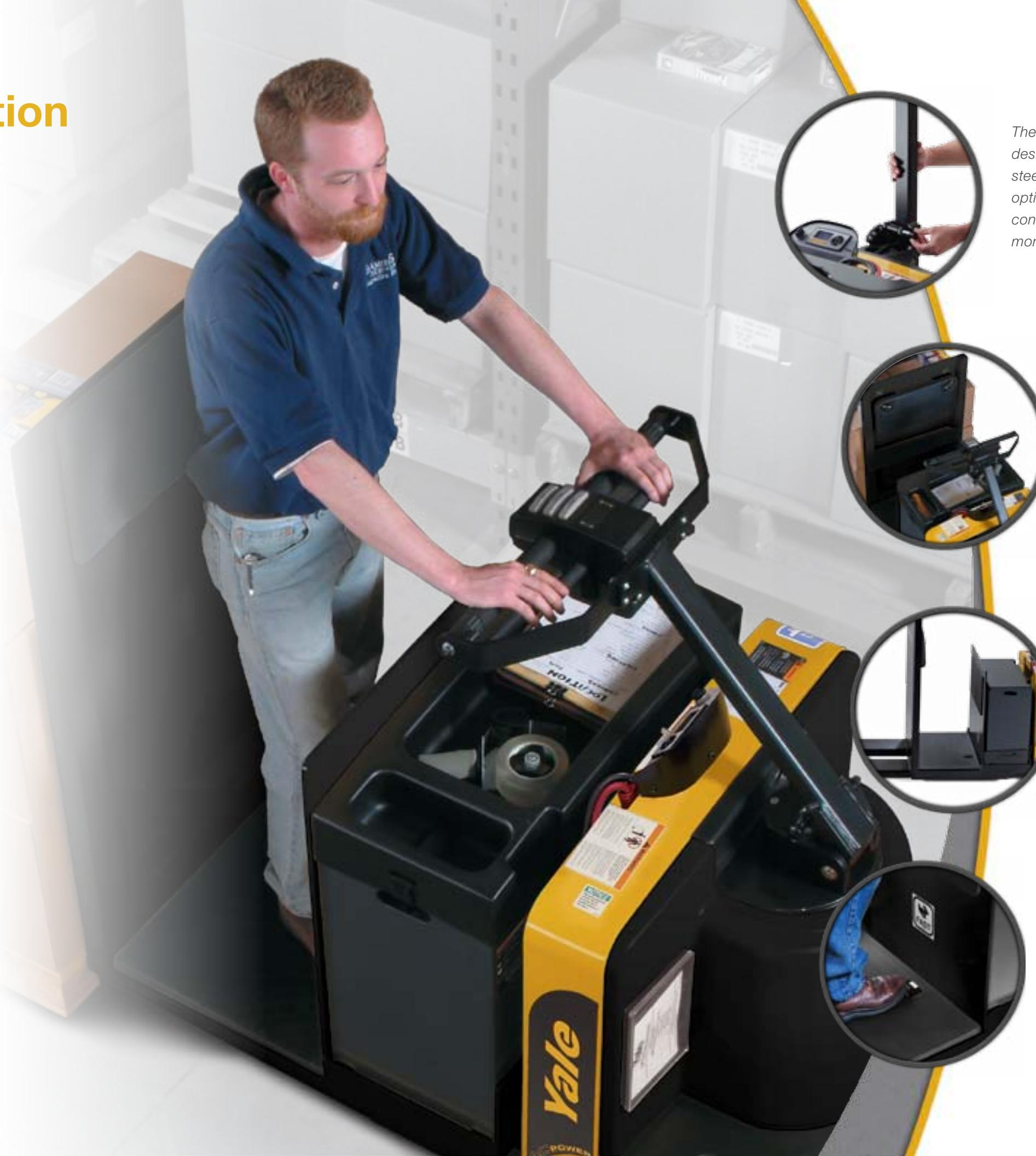
The vertically adjustable control handle design provides full control of travel, steering and horn while allowing optimum maneuverability. A 25"-wide control handle provides the operator more leverage for easy steering.
