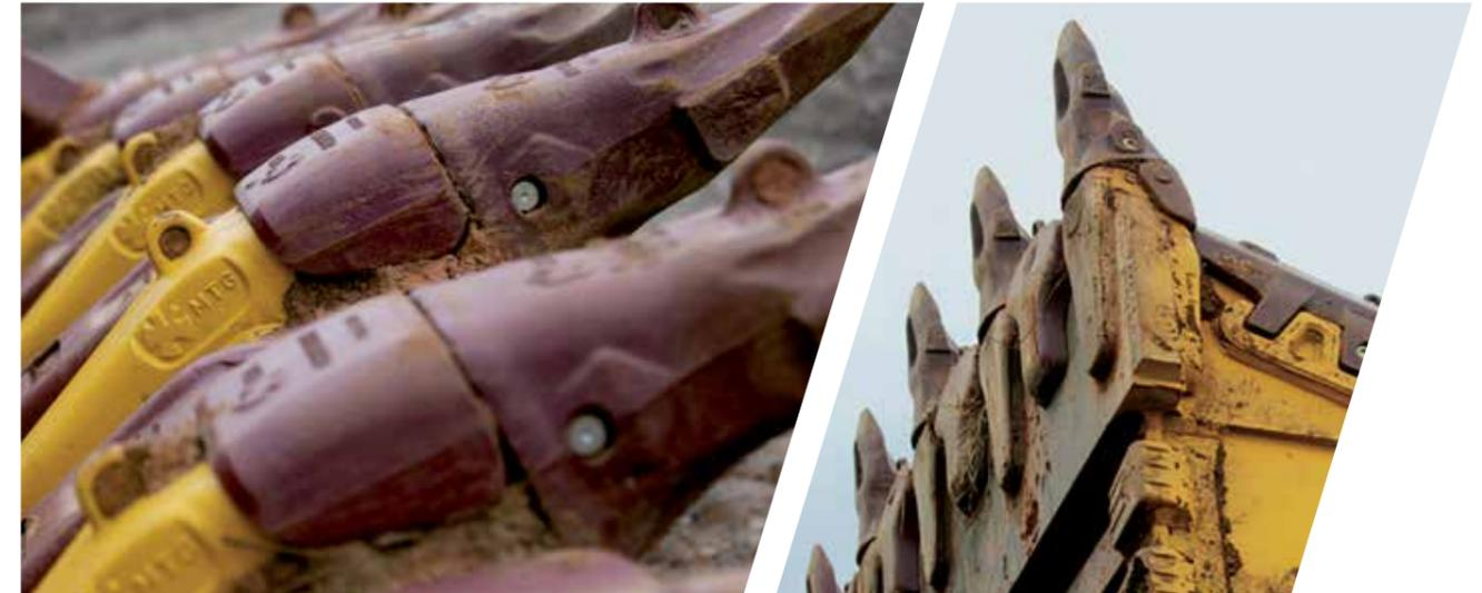
Teeth, adapters and shrouds specific for high levels of abrasion and impact.
