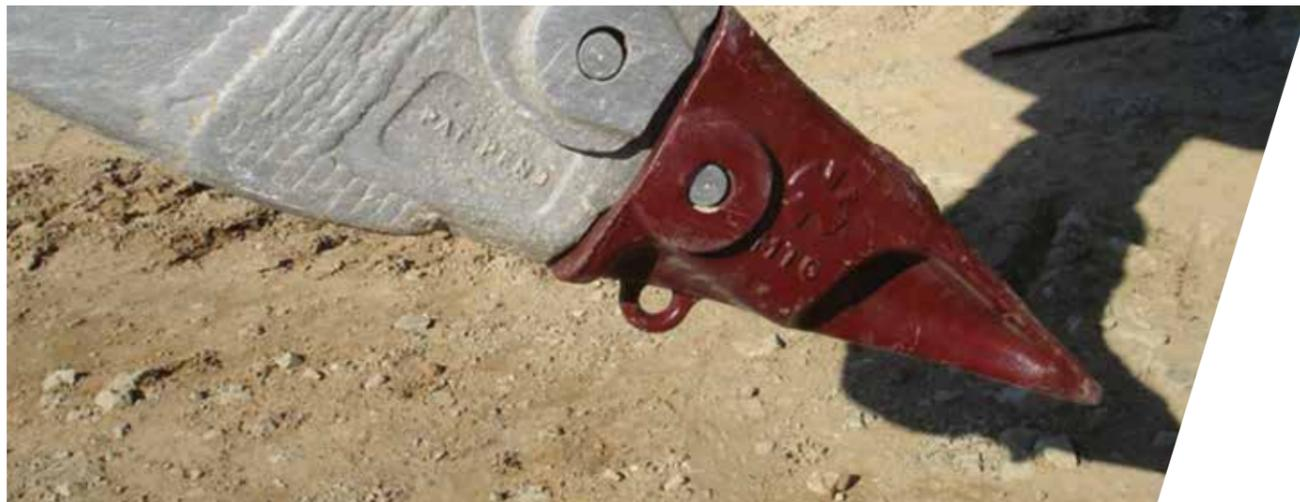
MTG Systems tooth for bulldozers working in Spain.
