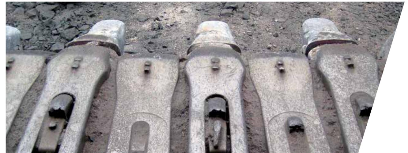
Close-up of a MTG Systems StarMet Rope Shovel adapter with a conventional locking system.
