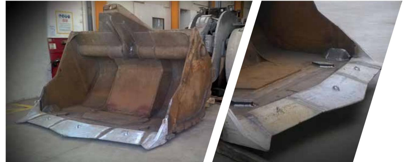
Bucket with LHD Lip System in underground copper mine.
