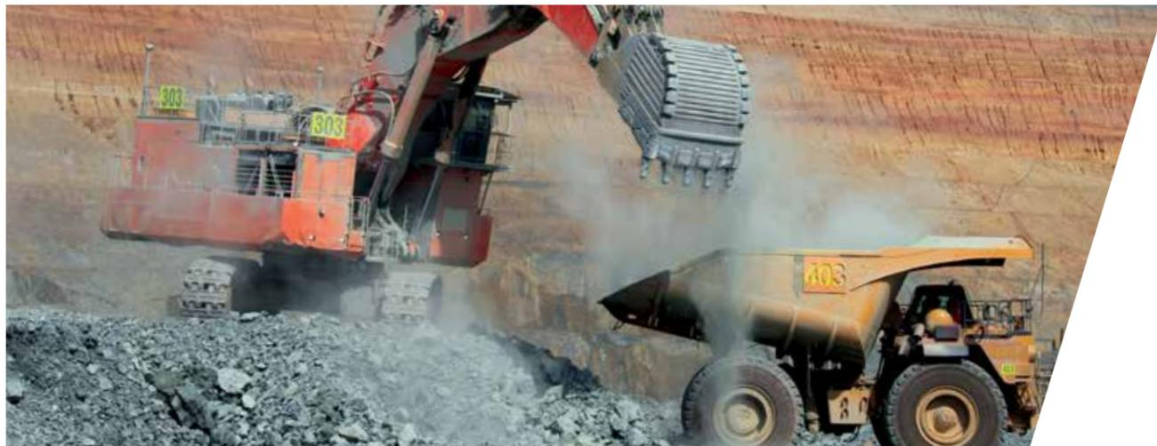
5 position excavator bucket working in a gold mine in Australia.
