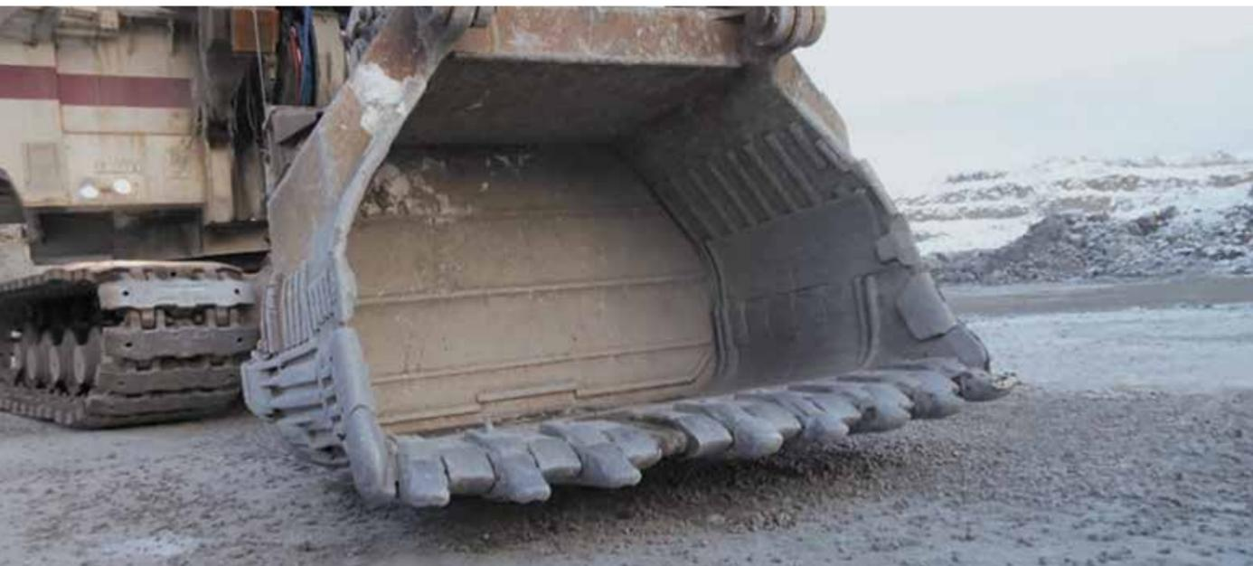
▶ MTG STARMET ROPE SHOVELS RANGE OF TEETH, ADAPTERS AND MECHANICAL SHROUDS
