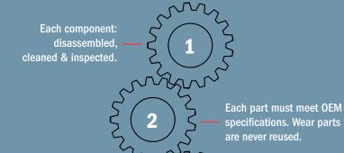
Scrapped parts are replaced with OEM parts originally used in component.
