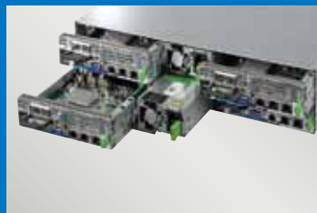
PRIMERGY CX250 S1 server node (installed in PRIMERGY CX400 S1)
