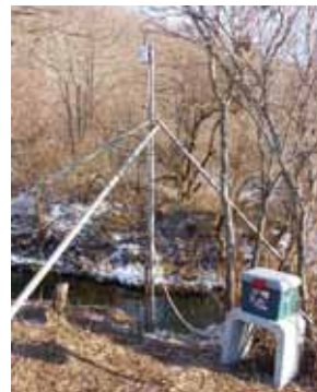
Multi-sensing unit installed at natural feeding ground for Japanese cranes
