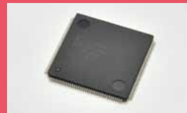
MB91580 series microcontroller with drive motor control functions for electric and hybrid vehicles
