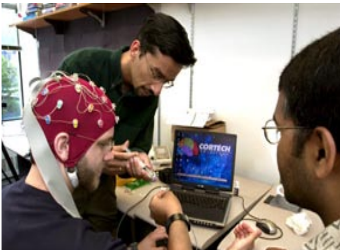
CSE professor Rajesh Rao and grad student Pradeep Shenoy hook UW medical student Jeff Longnion up to the Brain-Computer Interface (BCI). The goal of this research is to use brain signals to directly control computers and robotic devices.
