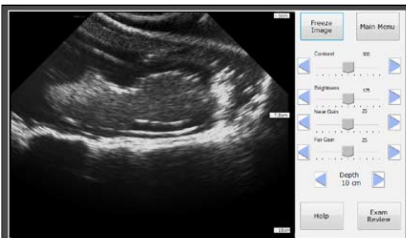
The team designed a simple interface specifically for midwives. Five slider bars adjust the image settings; four buttons control other functions, such as freezing the image or accessing the main menu.
