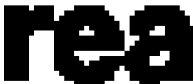
Figure 12: Ink spread and low resolution scans may cause several characters to become connected.
