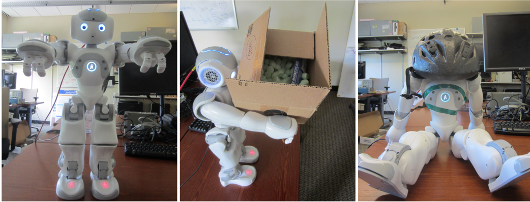
Figure 3-6: Left: Collecting weight data for the NAO without any load on it, and light data for a bright room. Center: Collecting weight data for the NAO holding a box filled with packing peanuts. Right: Collecting light data for the NAO wearing a helmet.
