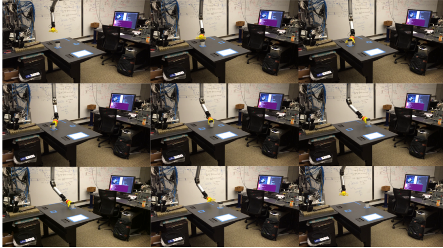
Figure 5: Demonstration of tabletop manipulation on hardware using kinematic planning. The task is to move the coffee cup from one location on the table to another.
